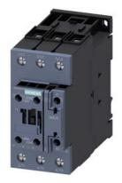
Power contactor, AC-3 80 A, 37 kW / 400 V 1 NO + 1 NC, 230 V AC, 50 Hz 3-pole, size S2 screw terminals
