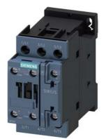
power contactor, AC-3 17 A, 7.5 kW / 400 V 1 NO + 1 NC, 230 V AC, 50 Hz, 3-pole, Size S0 screw terminal
