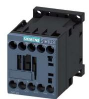
Power contactor, AC-3 12 A, 5.5 kW / 400 V 1 NO, 230 V AC, 50 / 60 Hz 3-pole, Size S00 screw terminal
