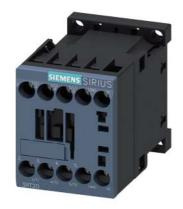
Power contactor, AC-3 9 A, 4 kW / 400 V 1 NO, 230 V AC, 50 / 60 Hz 3-pole, Size S00 screw terminal
