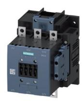
Power contactor, AC-3 185 A, 90 kW / 400 V AC (50-60 Hz) / DC operation 220-240 V UC Auxiliary contacts 2 NO + 2 NC 3-pole, Size S6 Busbar connections Drive: conventional screw terminal
